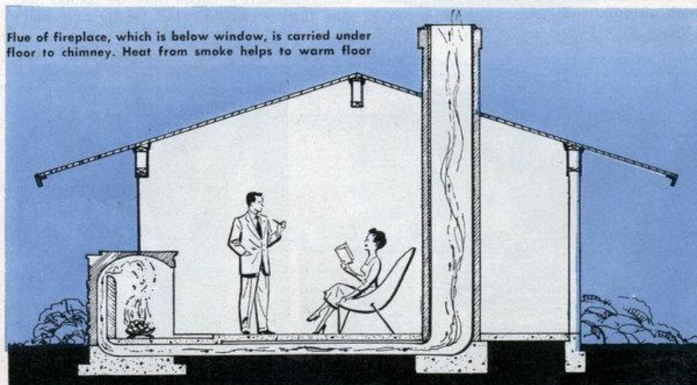
Flue of fireplace, which is below window, is carried under floor to chimney. Heat from smoke helps to warm floor
